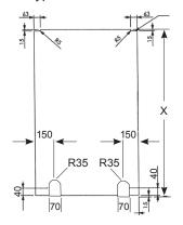
X = height of door which is finished opening height less 35mm
