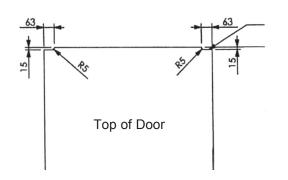
Details of top of Door. Notch Setout to accommodate top Channel Stops.
