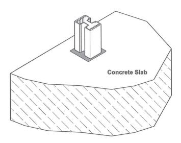
Design engineer must ensure deck can support a moment of 1.7 KNm applied at each post
