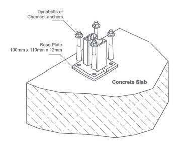
All fixings must engage into the structural slab
