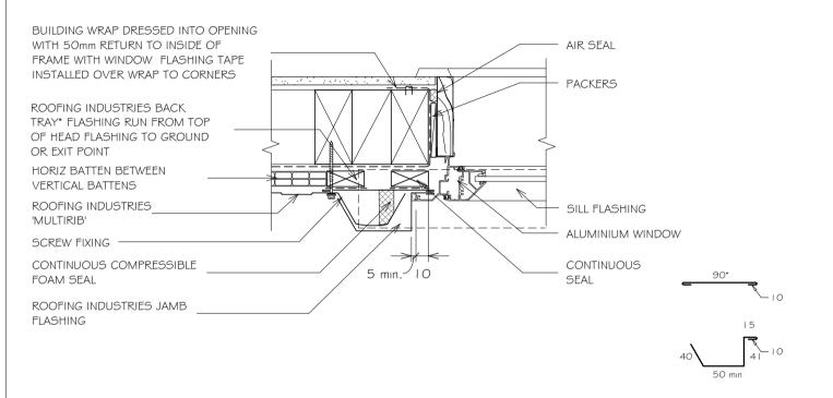
\* Back tray size may require to increase to ensure coverage at ends of head flashling. (Dimensions are indicative only)
