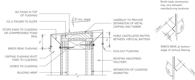
KICK-OUT at bottom edge of vertical flashing
