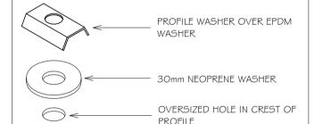
WHERE REQUIRED FOR EXPANSION OR WIND UPLIFT IN ROOFING APPLICATION
