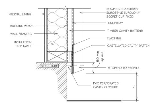
Detail Number: RI-EE50W005A Date drawn: 02/02/18 Scale: 1:5@ A4 1. FOR FIXING METHODS REFER TO SPECIFICATIONS. 2 THIS DETAIL TO BE CONFIRMED BY ROOFING INDUSTRIES TECHNICAL DEPT PRIOR TO USE. 3. ALLOW FOR SEPARATION FROM ANY CORROSIVE TIMBER TREATMENT 4. ALL DIMENSIONS SHOWN ON DRAWINGS ARE NOMINAL +/- 5mm 5. CASTELLATED TIMBER BATTEN OR APPROVED DRAINED BATTEN MAY BE USED WITH THIS SYSTEM MINIMUM
