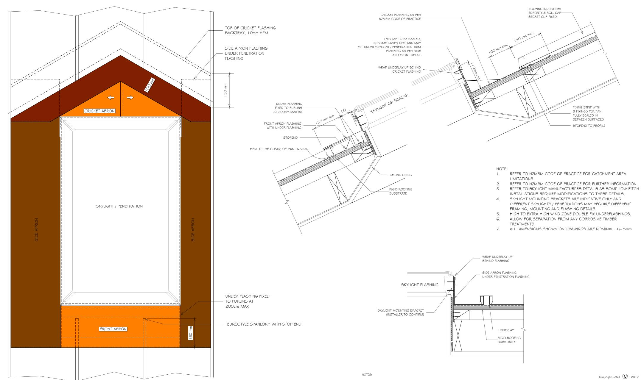
• These details are generally in compliance the NZ Metal Roof \$ Wall Cladding Code of Practice and in some cases specific details by 'Roofing Industries'. Eurostyle falls outsider the criteria of E2/AS I and this document is therefore not applicable.
