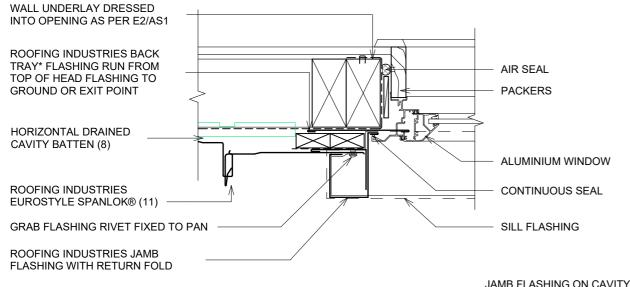
\* Back tray size may require to increase to ensure coverage at ends of head flashings. Turn down end of head flashing
