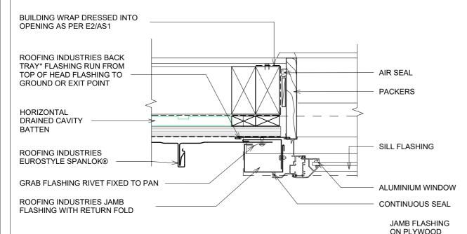
\* Back tray size may require to increase to ensure coverage at ends of head flashings. Turn down end of head flashing
