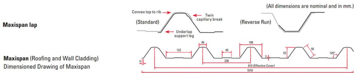
Acceptable Solution E2/AS1 provides for trapezoidal profile roofing with a minimum crest height of 19 mm and 210 mm maximum between crests.
