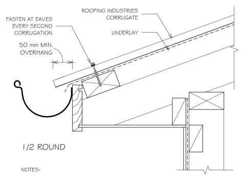
I. GUTTER APRON FLASHINGS MAY BE REQUIRED AS PER DRAWING RCROO4A
