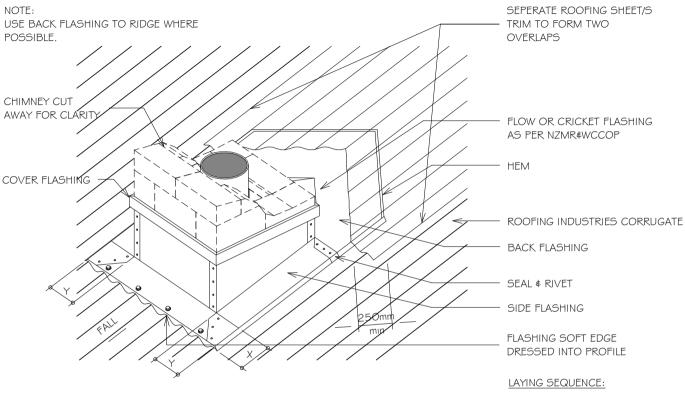
A. SOFTEDGE APRON,B. SIDE FLASHING,C. BACK FLASHING,D. COVER FLASHING (CHASED)
