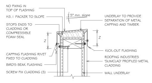
SLIMCLAD IS OUTSIDE THE SCOPE OF E2/AS I BUT MAYBE APPLICABLE FOR NON RESIDENTIAL BUILDINGS OR AS AN ALTERNATIVE SOLUTION KICK-OUT at bottom edge of vertical flashing
