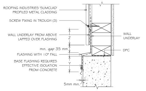
SLIMCLAD IS OUTSIDE THE SCOPE OF E2/AS I BUT MAYBE APPLICABLE FOR NON RESIDENTIAL BUILDINGS OR AS AN ALTERNATIVE SOLUTION KICK-OUT OPTION at bottom edge of vertical flashing
