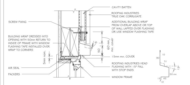
(Dimensions are indicative only) Turn down end of head flashing to jamb flashing
