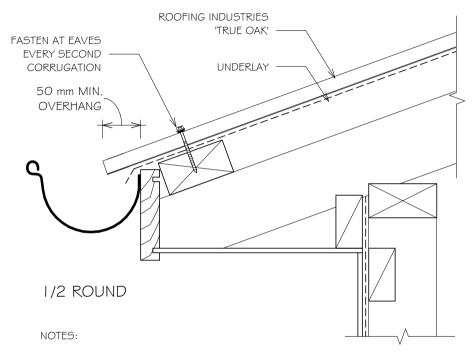
GUTTER APRON FLASHINGS MAY BE REQUIRED AS PER DRAWING RCRO04A
