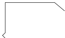
ROOFING INDUSTRIES BARGE FLASHING
