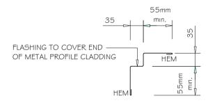
SEPARATION OF BATTEN AND METAL CLADDING ROOFING INDUSTRIES TRIMRIB' INTERNAL CORNER FLASHING COMPRESSIBLE FOAM SEALANT SCREW FIXING THROUGH BATTENS
