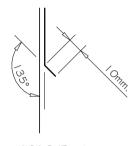
KICK-OUT at bottom edge of vertical flashing
