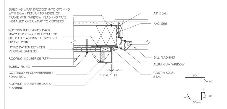
\* Back tray size may require to increase to ensure coverage at ends of head flashling. (Dimensions are indicative only) Turn down end of head flashing
