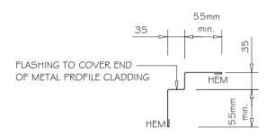
SEPARATION OF BATTEN AND METAL CLADDING ROOFING INDUSTRIES 'RT7' INTERNAL CORNER FLASHING COMPRESSIBLE FOAM SEALANT SCREW FIXING THROUGH BATTENS CAVITY BATTENS
