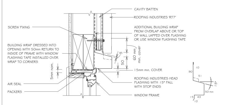
(Dimensions are indicative only) Turn down end of head flashing to jamb flashing Detail Number: RI-RRTW012A-1 Date drawn: 07/07/2017 Scale: 1:5@A4
