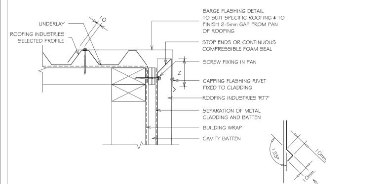
BIRD'S BEAK at bottom edge of vertical flashing Bırd's beak dimension may vary between manufacturing locations. SITE WIND ZONE MINIMUM (As per NZS3604) Z SITUATION I <sup>(1)</sup> 75mm<sup>(3)</sup>
