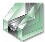
ThermoTech comprises two panels of glass separated by a metal spacer that is sealed with a primary vapour and a secondary seal to provide a hermetically sealed airspace. The spacer has a desiccant to prevent moisture forming inside the ThermoTech unit.
