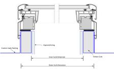
Timber used in construction of curb must not exceed 35mm to avoid interference with skylight operation and glass areas.
