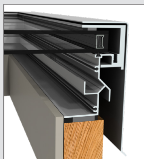
Frame detail with condensation collection.
