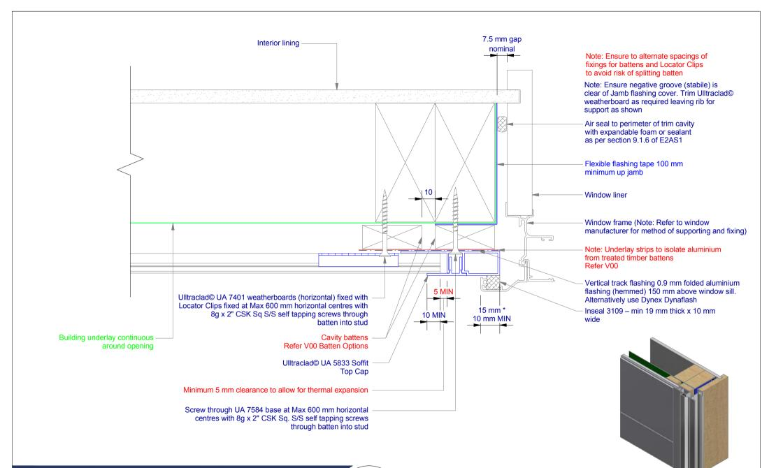
ULLTRACLAD ALUMINIUM CO LTD PO Box 98 843 Manukau City Auckland 2241 118 Wiri Station Road Wiri 2104 New Zealand TL 09 262 6262 Ext. 814 Mob 021 541 563 www.ulltraclad.co.nz © ULLRICH ALUMINIUM - All Rights Reserved Window Jamb on Cavity UA 7401 INFINITY BOARD
