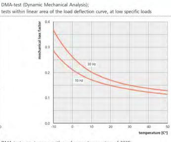
DMA-tests; mastercurve with a reference-temperature of 21°C; tests within the linear area of the load deflection curve, at low specific li
