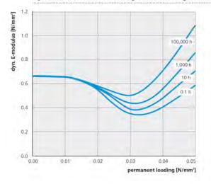
increase in deformation under consistent loading **parameter:** permanent loading shape factor q=3
