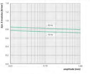
preload at static load limit; shape factor: q=3, thickness of material 25 mm
