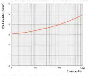
dependency on loading velocity shape factor: q=3, thickness of material 25 mm
