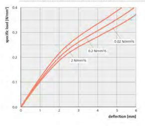
tests within the linear area of the load deflection curve, at low specific loads
