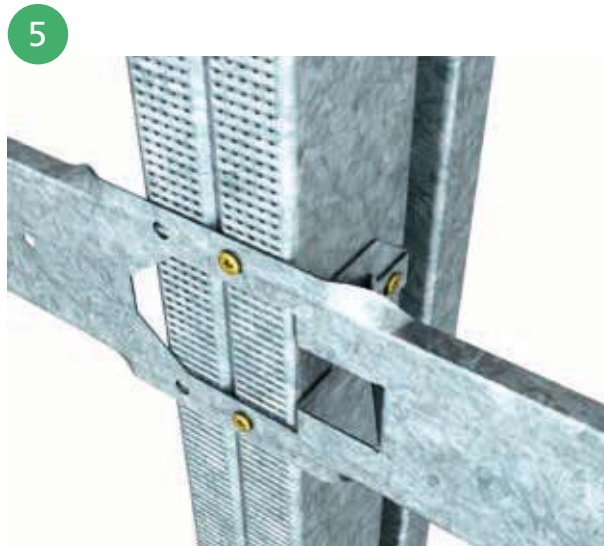
■ FAST-FIX NOGGING INSTALLED INTO RONDO QUIET STUD® NOTE: Ensure Rondo QUIET STUD® is installed in the correct orientation to ensure the FAST-FIX Nogging is only fitted to the wide web element.
