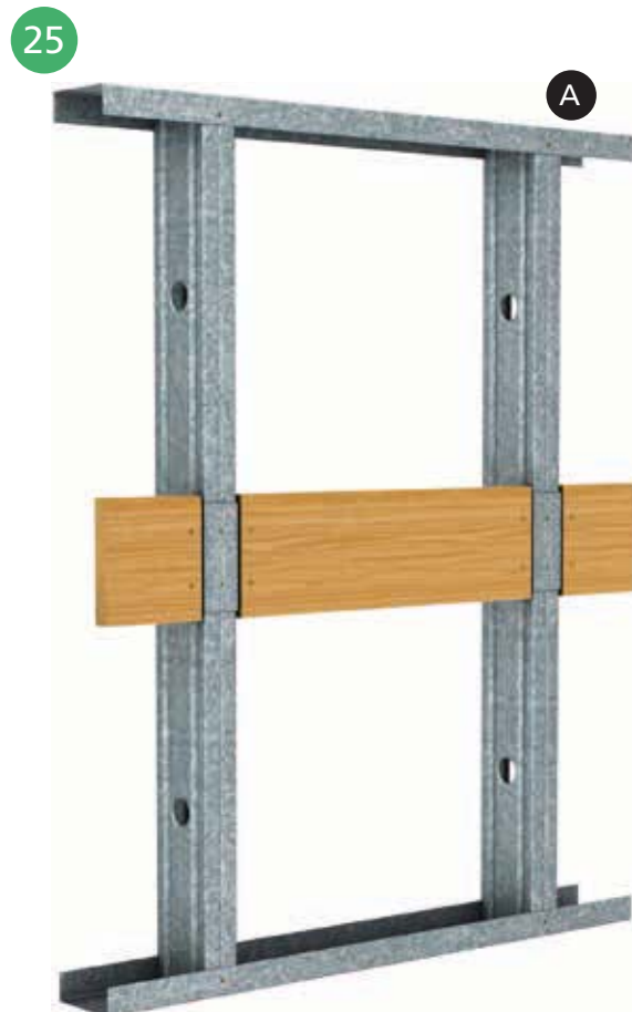
■ TIMBER NOGGINGS NOTCHED TO FIT BETWEEN STUD WEBS
