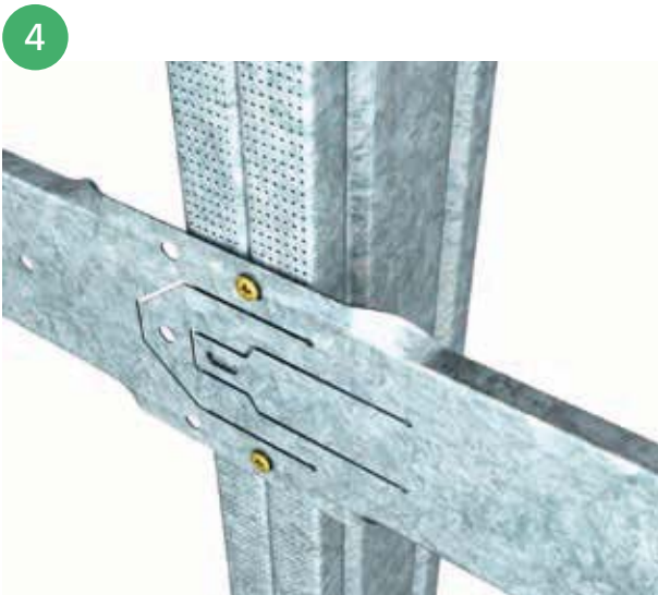
■ FAST-FIX NOGGING INSTALLED INTO RONDO STEEL STUD USING FACE-FIX x 2 SCREWS METHOD
