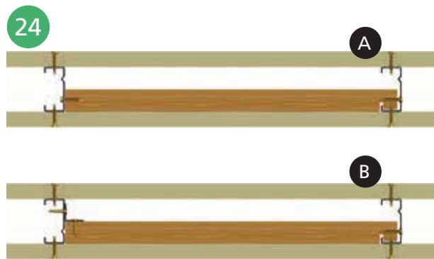
■ TIMBER NOGGINGS NOTCHED TO FIT BETWEEN STUD WEBS
