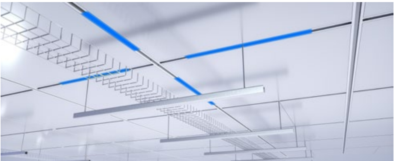
Load Case Zone 3 - 60kg maximum anywhere outside of zone 2, where load must be in adjacent bays
