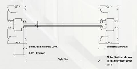
Note: Edge cover is defined as fully dupporting the glass - glazing gasket or wedge extending beyond the frame backing should not be considered as part of the edge cover.
