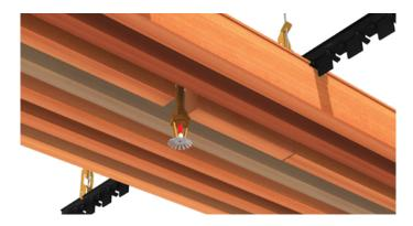
**4.** Keep in mind that special features, such as air-conditioning vents, may require extra rails and clips to support the cut timber.
