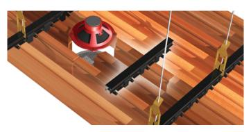
**5.** Ensure that any smaller joins are properly supported with a short TCR rail and clips covering the adjacent profiles.
