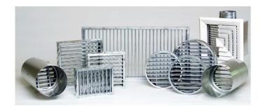
BOSS Intumescent Fire Dampers allow the bi-directional movement of air through fire rated walls and floors. In a fire situation the slats in the damper intumesces and swells to many times the original size, closing the damper and forming a solid fire barrier. They are simple to install, easy to identify, and economical to maintain.
