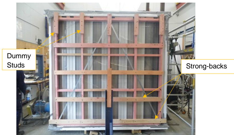
Figure 3. Initial test set up of first three tested specimens shown in pressure box
