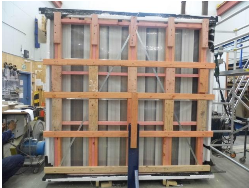
Figure 4. Augmented test set up of first three tested specimens with additional timber and extended strong-backs
