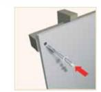
Mark out and drill fixing holes. Insert toggle.
