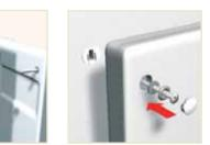
Align and engage the If fixing bolt in the threaded toggle bar with washers engaged. The flat fender washer is to be inserted underneath the finishing washer. Finally, insert the snap-fit plastic covers in each fixing port.
