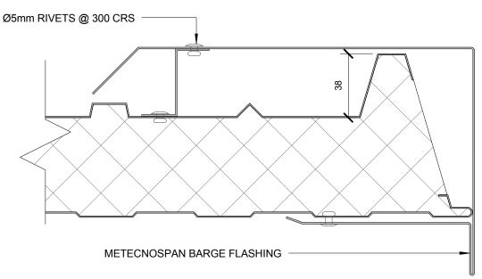
SIDE BARGE FLASHING DIMENSIONS
