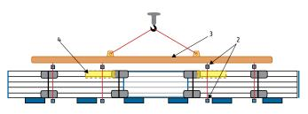
Fig. 8. Unloading of Panels of > 8.0 m: 3. Spreader Beam; 4. Strap-down Corner Angles.
