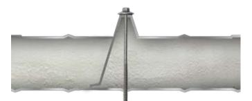
Composite panels are interlocked together.
