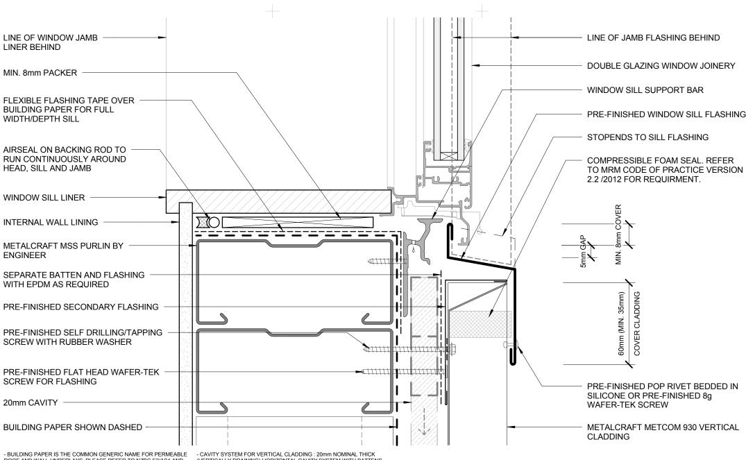
CAVITY SYSTEM FOR VERTICAL CLADDING: 20mm NOMINAL THICK (VERTICALLY DRAINING) HORIZONTAL CAVITY SYSTEM WITH BATTENS AS APPLICABLE TO SUPPORT CLADDINGS & FLASHINGS TO NZBC.
