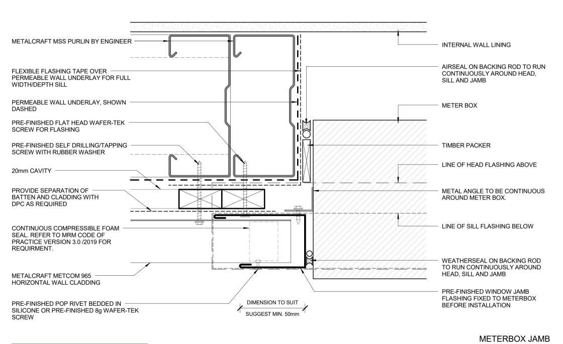
All details are to be used for indicative purposes only and the designer should consult both the MRM code of practice version 3.0 / 2019, E2 and all other relevant building codes Details of the supporting mechanisms are indicative only. Compliance of the supporting mechanisms is the responsibility of the designer. Construction detail can vary for wall cladding. The underlay is detailed as a
