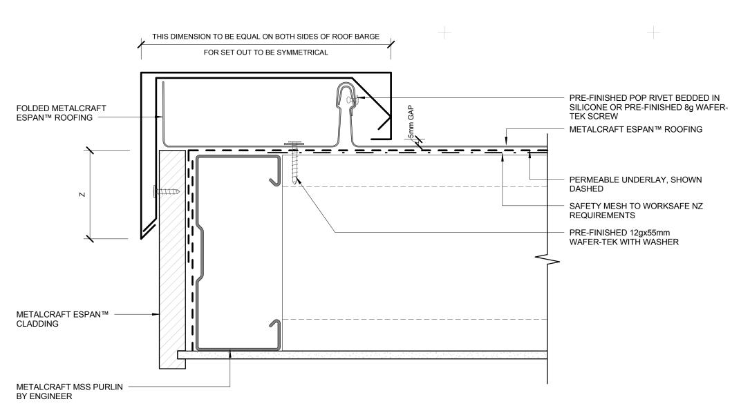
ACCEPTABLE SOLUTION AS PER E2/ASI SITUATION 1 SITUATION 3 1. ALL ROOF PITCHES IN VERY HIGH WIND ZONE 2. LOW, MEDIUM AND HIGH WND ZONES WHERE ROOF PITCH ≤ 10° 1. LOW, MEDIUM, HIGH WIND ZONES WHERE ROOF PITCH ≥ 10° 1.ALL ROOF PITCHES IN EXTRA HIGH WIND ZONE. AT LEAST TWO CRESTS AT LEAST TWO CRESTS AT LEAST TWO CRESTS MIN. 50mm MIN. 70mm MIN. 90mm
