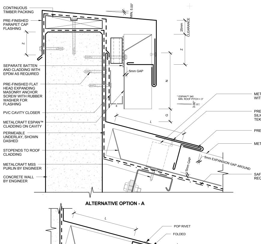
ACCEPTABLE SOLUTION AS PER E2/ASI SITUATION 1 SITUATION 3 1. ALL ROOF PITCHES IN VERY HIGH WIND ZONE 2. LOW, MEDIUM, & HIGH WIND 1. LOW, MEDIUM, HIGH WIND ZONES, WHERE ROOF PITCH ≥ 10° 1. ALL ROOF PITCHES IN EXTRA HIGH WIND ZONE MIN. 35mm MIN. 35mm G MIN. 35mm MIN. 75mm MIN. 75mm MIN. 75mm MIN. 200mm (EXCLUDING ANY SOFT EDGE OR MIN. 200mm (EXCLUDING ANY SOFT EDGE OR TURN-DOWN TO ROOFING) (EXCLUDING ANY SOFT EDGE OR TURN-DOWN TO ROOFING) TURN-DOWN TO ROOFING) MIN. 90mm
