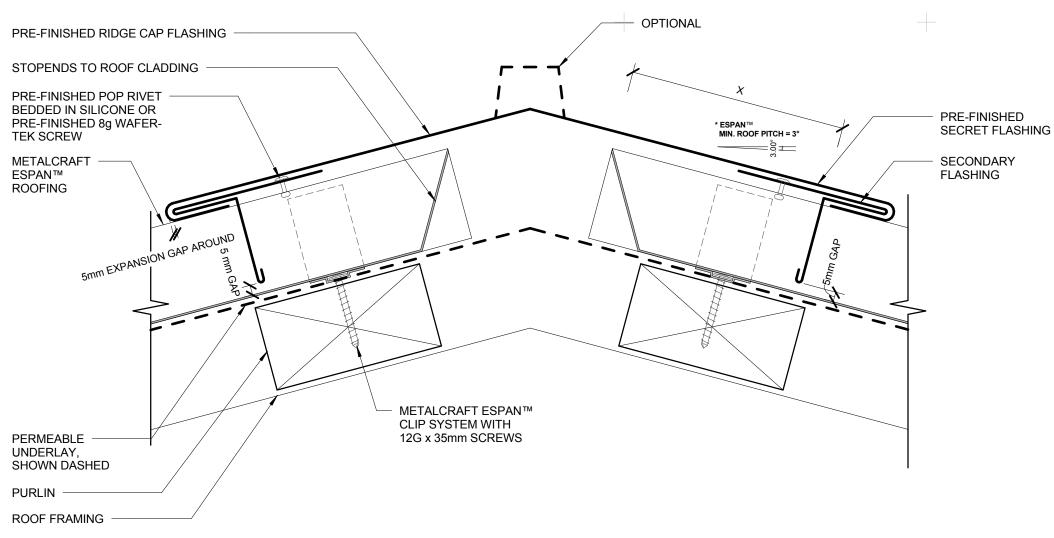
ACCEPTABLE SOLUTION AS PER E2/AS1 SITUATION 1 SITUATION 2 SITUATION 3 1. LOW, MEDIUM, HIGH WIND ZONES 2. ROOF PITCH ≥ 10° 1. FOR ALL ROOF PITCHES IN EXTRA HIGH WIND ZONES 1. ALL ROOF PITCHES IN VERY HIGH WIND ZONE
