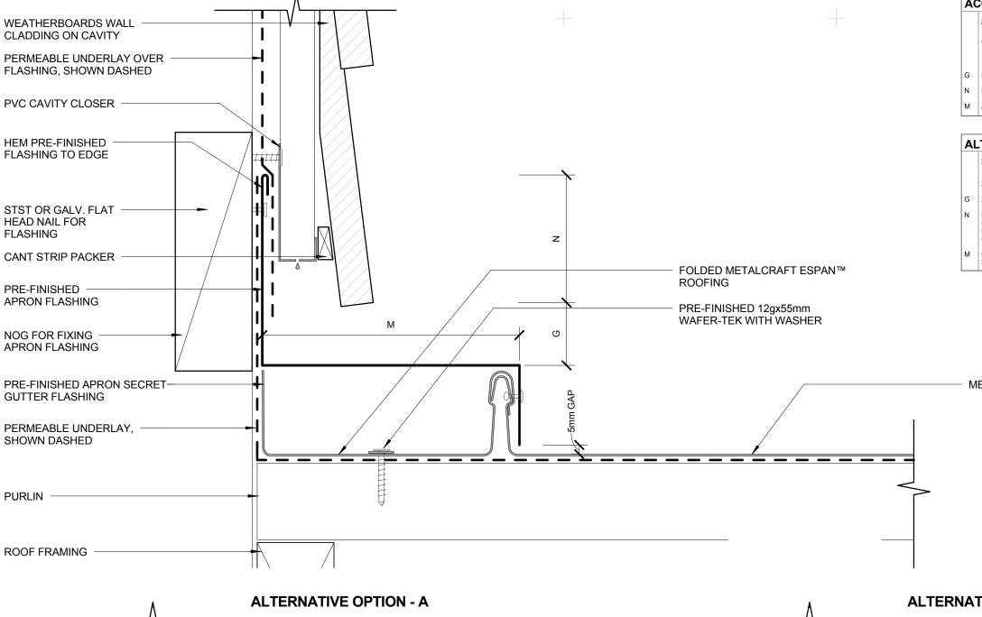
ACCEPTABLE SOLUTION AS PER E2/ASI SITUATION 3 1. LOW, MEDIUM, HIGH WIND ZONES, WHERE ROOF PITCH ≥ 10° 1. ALL ROOF PITCHES INVERY HIGH 1. ALL ROOF PITCHES IN EXTRA WIND ZONE
