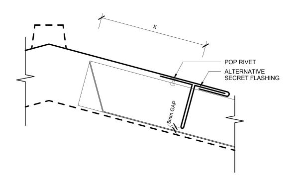
RIDGE FLASHING RESIDENTIAL ROOFING Espan 340™ / 470™ Rev: R0 Sheet **01 / 20** Date 2018 Reference RREP
