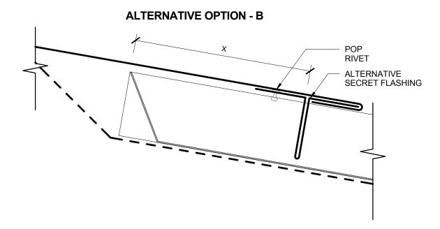
**ROOF - CHANGE PITCH** Espan 340™ / 470™ RESIDENTIAL ROOFING Rev: R0
