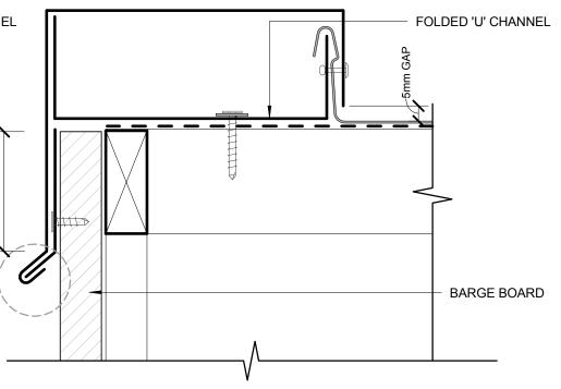
BARGE FLASHING RESIDENTIAL ROOFING Espan 340™ / 470™
