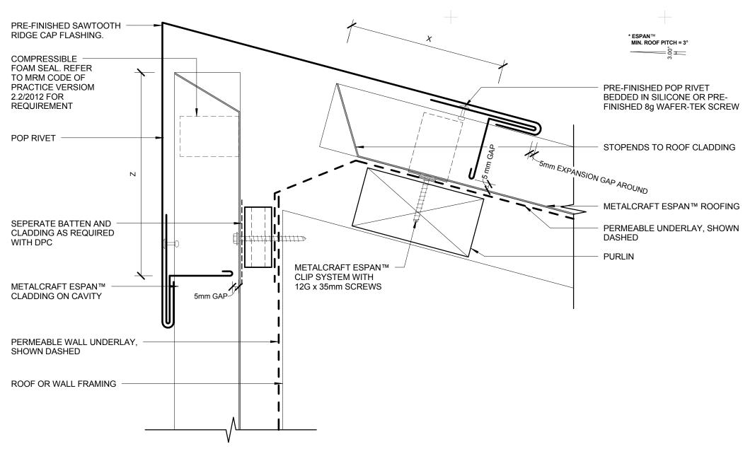
**ACCEPTABLE SOLUTION AS PER E2/ASI** SITUATION 1 **SITUATION 3** 1. ALL ROOF PITCHES INVERY HIGH WIND ZONE 2. LOW, MEDIUM AND HIGH WIND ZONES WHERE ROOF PITCH ≤ 10° 1. LOW, MEDIUM, HIGH WIND ZONES, WHERE ROOF PITCH ≥ 10° 1.ALL ROOF PITCHES IN EXTRA HIGH MIN. 200mm MIN. 130mm (EXCLUDING ANY SOFT EDGE OR (EXCLUDING ANY SOFT EDGE OR TURN-DOWN TO ROOFING) MIN. 200mm (EXCLUDING ANY SOFT EDGE OR TURN-DOWN TO ROOFING) TURN-DOWN TO ROOFING)
