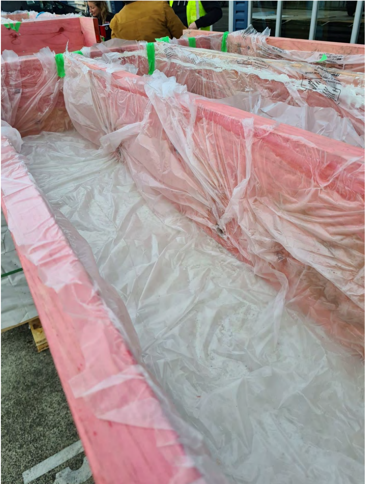
Photo 1: Fixing of 0.4 mm plastic very loosely to frame to allow movement under the water
