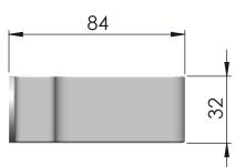
**NOTE: Fixing recommendations**Stainless Steel, grade 304 8g screw with neutral coloured washer to go between clip and wall.
