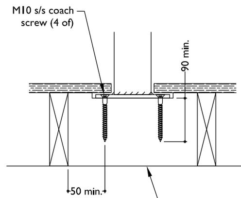
note: fixings to be 50 min. from the end and 25 min. from the edge of the timber
