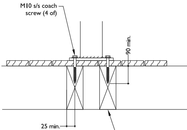
note: fixings to be 50 min. from the end and 25 min. from the edge of the timber
