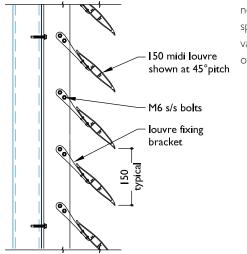
note: pitch (angle) and spacing of louvres can vary and are set at time of manufacturing
