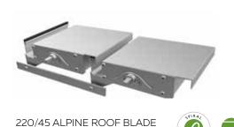
• Due to the extended span of this blade, the 220/45 Alpine Louvre has a 20x3 End Cap Connecting Bar fitted below the blade to eliminate any individual blade movement in extreme conditions.
