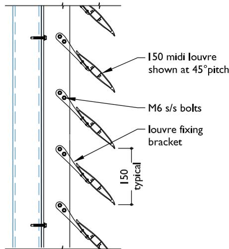
note: pitch (angle) and spacing of louvres can vary and are set at time of manufacturing
