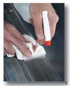
Simply clean with a solution of water and isopropyl alcohol and wipe dry.
